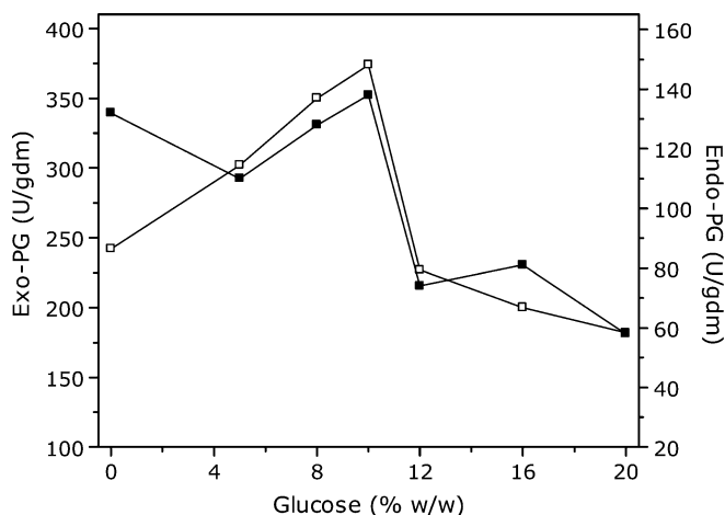
Fig. 6 Variation of exo-PG (open square) and endo-PG (filled square) activities with the initial concentration of glucose in wheat-bran solid medium containing 6% (w/w) citric pectin (48 and 72 h of process, respectively)
